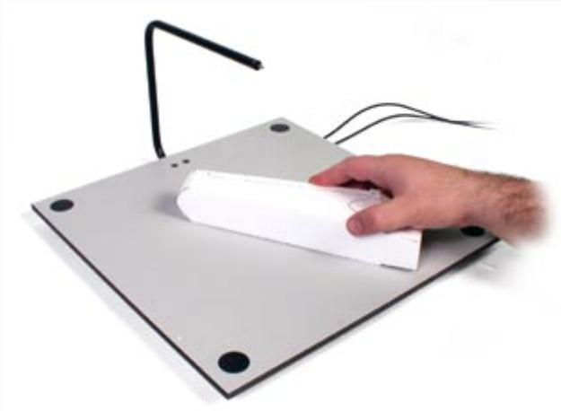
2. Use a hot wire foam cutter to roughly shape the blank:
