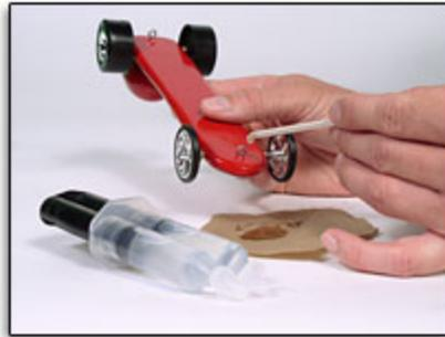
4. Roll test the car on a smooth, horizontal surface. The car should roll freely, and the wheels should spin without restriction. Make adjustments if necessary.
