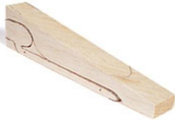
c. Set the blank assembly upright and cut out the top view.
