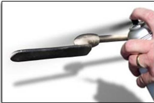
1. Insert a 2-foot length of 5/8" hardwood dowel into the power plant housing of the car body. This makes a very convenient handle for turning the body to paint it from all angles. Pitsco also makes a racecar paint stand for this purpose.
