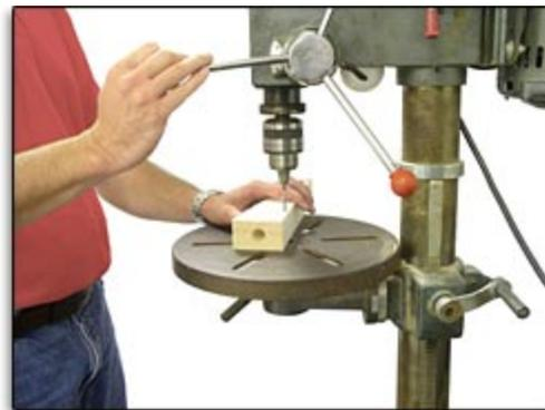
2. Lay the car blank on its side and drill the axle holes. Axle holes should be drilled perpendicular to the car's longitudinal axis in order for the car to roll freely and straight down the track. A drill press is highly recommended because it makes drilling perpendicular holes a cinch.
