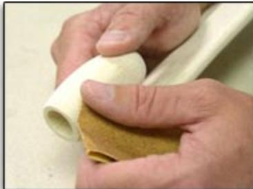
Use sandpaper to remove unwanted bumps and irregularities from the body. Use progressively finer grit paper as you go. For example, you might start with 80-grit paper (very coarse, removes a lot of material) and progress to 220-grit (fine paper for smoothing surfaces).
